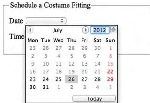
Figure 8-8. Opera displays a calendar interface when a date field receives focus. A user can select a year, month, and day with a few clicks and the browser will automatically enter the date in a machine-readable format.
