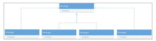
Selecting the correct strategy to use can be done in a number of different ways. The simplest method is to select the strategy statically. This can be done through a configuration variable or even hard coded. This approach is best for times when the strategy changes infrequently or is specific to a single customer or user.
