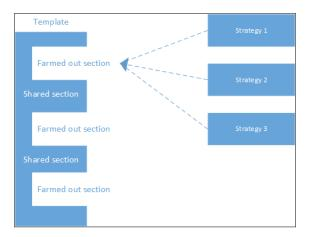
The template class implements parts of the algorithm and leaves other parts as abstract to later be overridden by classes which extend it. The inheritance hierarchy can be several layers deep, with each level implementing more and more of the template class.
