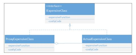
As you can see, the proxy mirrors the interface of the actual instance. It is substituted in for the instance in all the clients and, typically, wraps a private instance of the class. There are a number of places where the proxy pattern can be of use:
