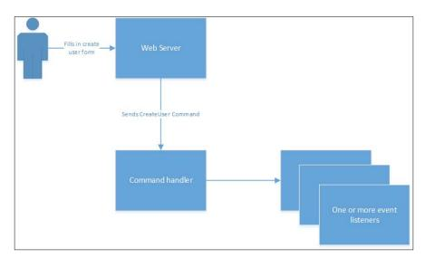
Here a user enters data into a form and submits it. The web server takes in the input, validates it and, if it is correct, creates a command. The command is now sent to the command handler. The command handler performs some action, perhaps writes to a database, it then publishes an event that is consumed by a number of event listeners. These event listeners might send confirmation e-mails, notify system administrators, or any number of things.
