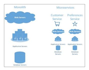
Applications are written more by composing services than by writing singular monolithic applications. The UI of an application can even be created by asking a number of services to provide visual components to be slotted into a composite UI by some form of composing service.
