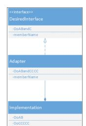
The class diagram for an adapter is very simple as can be seen here:
