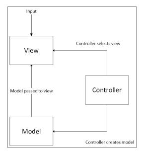
The preceding diagram shows the relationship between the three components in MVC.
