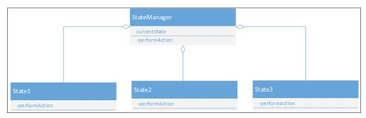
Splitting state into a class per state allows for much smaller blocks of code to debug and makes testing much easier.
