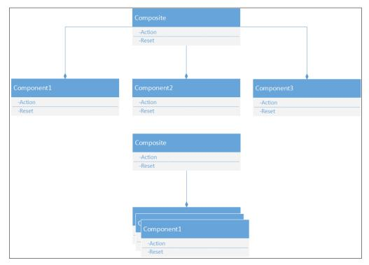
In the first one, the composite component is built from a fixed number of a variety of components. The second component is constructed from a collection of indeterminate length. In both cases the components contained within the parent composition could be of the same type as the composition. So a composition may contain instances of its own type.
