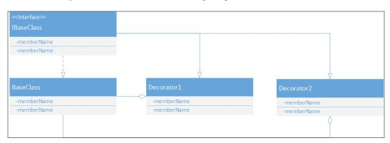
This allows for very granular control over which methods are altered by the decorator and which remain as mere pass-through. Let's take a look at an implementation of the pattern in JavaScript.
