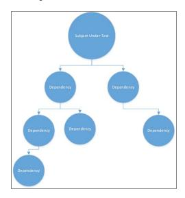
We need to find a way to isolate the class under test so that we don't have to recreate all the dependencies, including the network. We can think of this approach as adding bulkheads to our code. We will insert bulkheads to stop tests from flowing over from one class to many. These bulkheads are similar to how oil tankers maintain separation to limit the impact of spills and maintain weight distribution as can be seen here:
