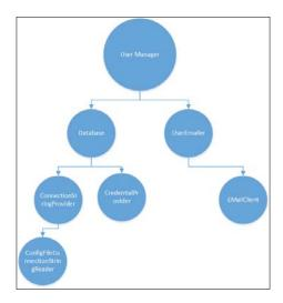
In more statically typed languages such as C# or Java, dependency injection frameworks are commonplace. They usually work by using reflection, a method of using code to extract structural information from other code. When building the container, one specifies an interface and one or more concrete classes that can satisfy the interface. Of course using interfaces and reflection to perform dependency injection requires that the language support both interfaces and introspection.
