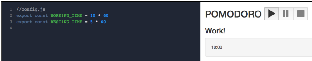
Changing the configuration for the amount of working time will immediately affect the Pomodoro application view
