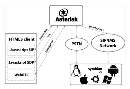
As you can see, **HTML5 client** can interact with a VoIP platform using WebRTC and a SIP module (**JavaScript SIP** in the diagram).
