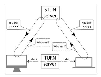
The schema in the following diagram depicts the data flow while using a TURN server:
