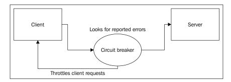
For the server, having the number of clients drop off as failures pile up allows for some breathing room to recover. The chances of a storm of requests coming in and keeping the system down is minimized.
