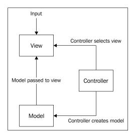
The preceding diagram shows the relationship between the three components in MVC.
