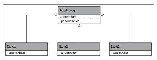
Splitting state into a class per state allows for much smaller blocks of code to debug and makes testing much easier.
