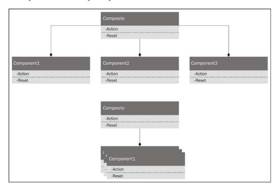
The preceding class diagram contains two different ways to build a composite. In the first one, the composite component is built from a fixed number of a variety of components. The second component is constructed from a collection of indeterminate length. In both cases, the components contained within the parent composition could be of the same type as the composition. So a composition may contain instances of its own type.
