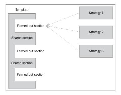
The template class implements parts of the algorithm and leaves other parts as abstract to be overridden later by classes that extend it. The inheritance hierarchy can be several layers deep, with each level implementing more and more of the template class.
