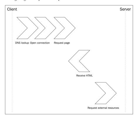
Connections to the web server should be limited to avoid paying the connection setup costs repeatedly. This brings us to our first concept: combining files.
