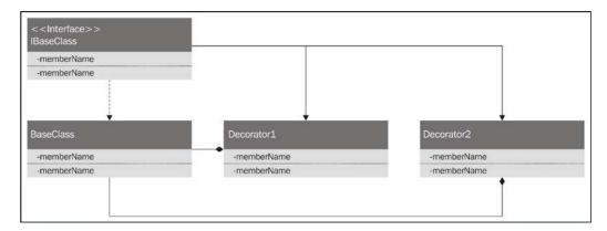
This allows for very granular control over which methods are altered by the decorator and which remain as mere pass-throughs. Let's take a look at an implementation of the pattern in JavaScript.
