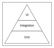
Unit tests form the foundation of the pyramid. They are the most numerous, the easiest to write, and the most granular in the errors they give. An error in a unit test will allow you to find the individual method that has an error in it. As we move up the pyramid, the number of tests falls along with the granularity, while the complexity of each test increases. At a higher level, when a test fails, we might only be able to say *there is an issue with adding an order to the system*.
