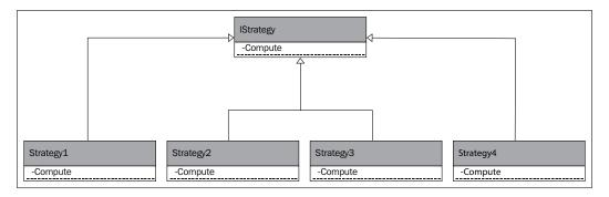
Selecting the correct strategy to use can be done in a number of different ways. The simplest method is to select the strategy statically. This can be done through a configuration variable or can even be hardcoded. This approach is best for times when the strategy changes infrequently or is specific to a single customer or user.
