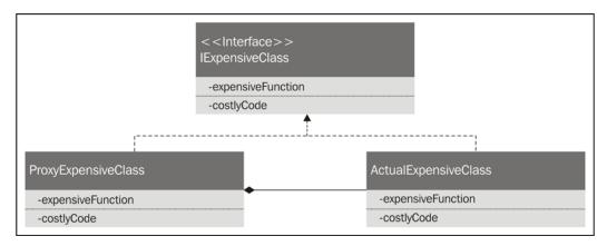
As you can see, the proxy mirrors the interface of the actual instance. It is substituted for the instance in all the clients and, typically, wraps a private instance of the class. There are a number of places where the proxy pattern can be of use:
