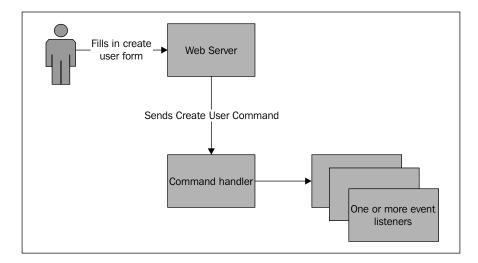
Here, a user enters data into a form and submits it. The web server takes in the input, validates it, and, if it is correct, creates a command. The command is now sent to the command handler. The command handler performs some action, perhaps writing to a database; it then publishes an event that is consumed by a number of event listeners. These event listeners might send confirmation e-mails, notify system administrators, or any number of things.
