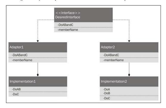
The adapters shown in the preceding diagram sit between the implementation and the desired interface. They modify the implementation to fit in with the desired interface.
