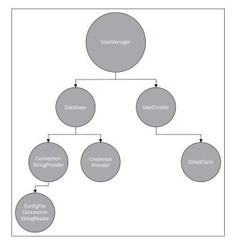
A dependency injection framework handles the responsibility of constructing objects. On application setup, the dependency injection framework is primed with a combination of names and objects. From this, it creates a registry or a container. When constructing an object through the container, the container looks at the signature of the constructor and attempts to satisfy the arguments on the constructor.
